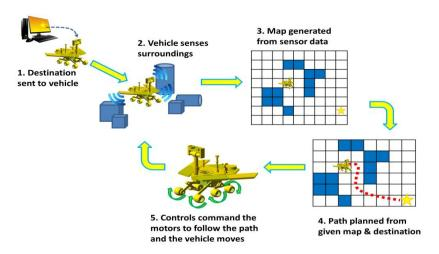
Figure 1: Example of Autonomous Vehicle Operation
