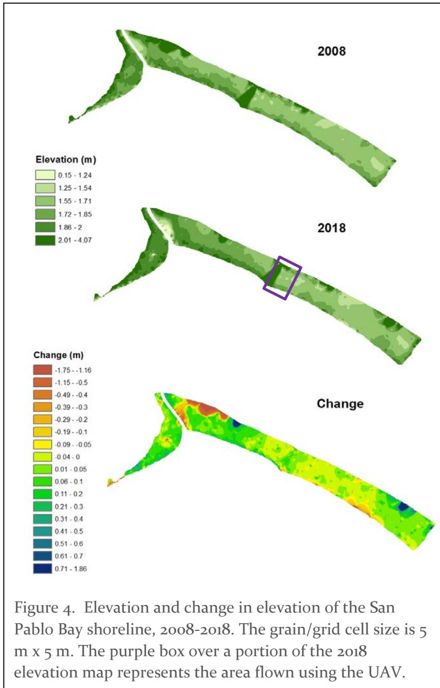
Figure 4. Elevation and change in elevation of the San Pablo Bay shoreline, 2008-2018. The grain/grid cell size is 5 m x 5 m. The purple box over a portion of the 2018 elevation map represents the area flown using the UAV.
