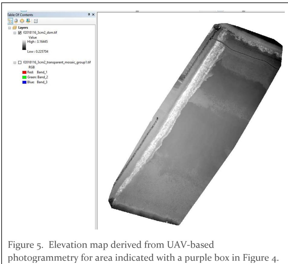
Figure 5. Elevation map derived from UAV-based photogrammetry for area indicated with a purple box in Figure 4.
