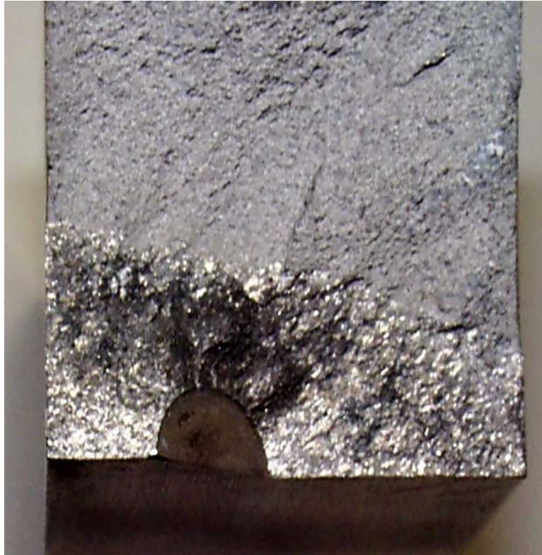
Figure 28. Final observed crack shape. The shiny fracture surface is the fatigue crack; duller surface is fast fracture, Example 14.
