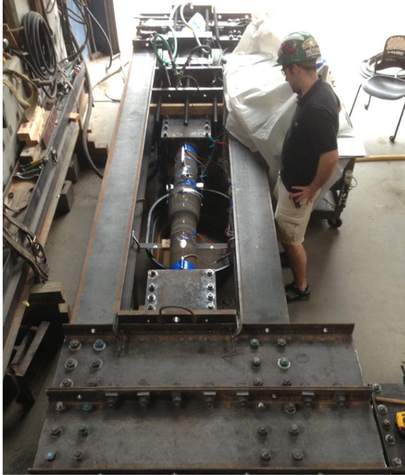
Figure 3. Photo of 6 in. Pipe Compression Test
