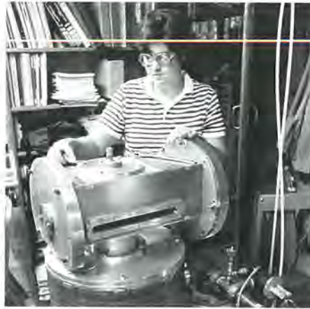
Studies of an advanced switching technique for pulsed-power generators are being conducted by Lynne Adler, a graduate student working with Professor Hammer. Devices such as the “plasma opening switch” Adler is working on are expected to be key to the development of ion-beam generation technology for light-ion fusion.
